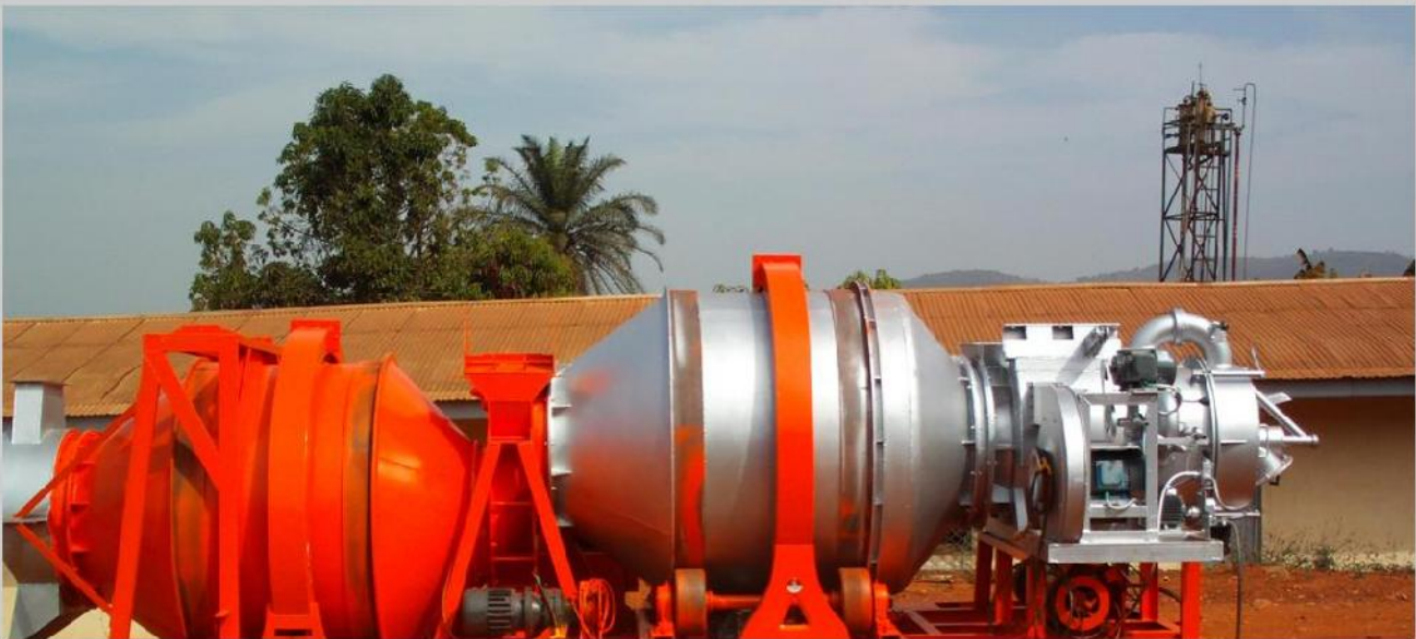
HRODC_AP15 10TPH Asphalt Plant — Part Installed Without Options
